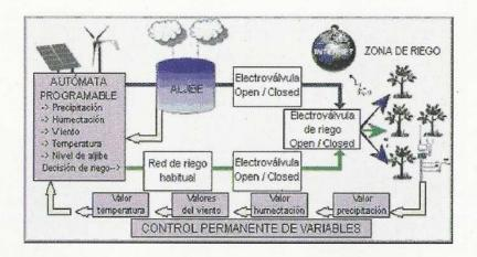
Such decisions concerning irrigation have been supplemented by programming the system so as to inhibit or stop the water supply when the data provided by the weather station advise against irrigation, on the basis of strict efficiency parameters (excessive wind speed, presence of rain, above-normal levels of moisture in the soil...).
